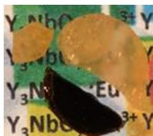
**Figure 1.**  $Y_3NbO_7:Eu^{3+}$  samples sintered by SPS, before (black specimen) and after (lighter specimens) post-annealing.
